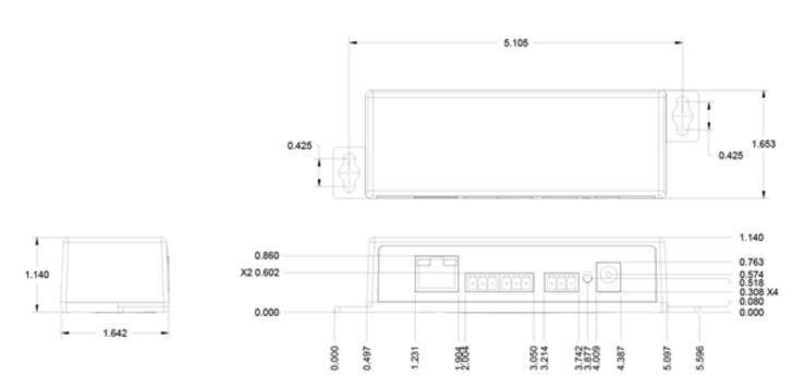
Figure 10 - AXP2O Dimensional Drawings
