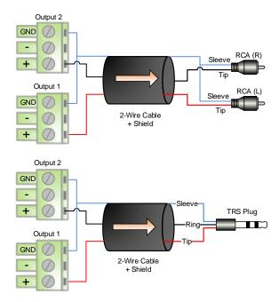
Figure 12 - AXP2O to Unbalanced Input Wiring Guide
